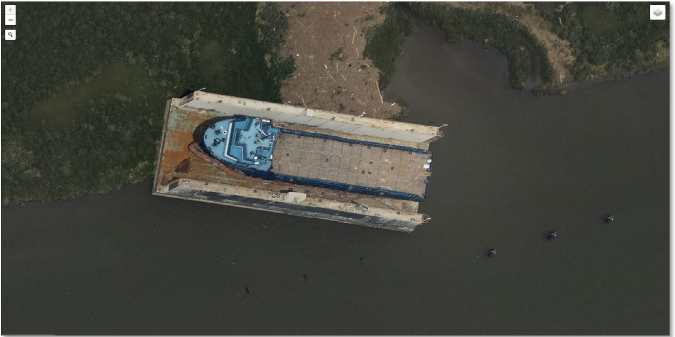
Figure 4: An AHTS (anchor handling tug supply) vessel swept ashore in the Port Fourchon area on a floating dock.
